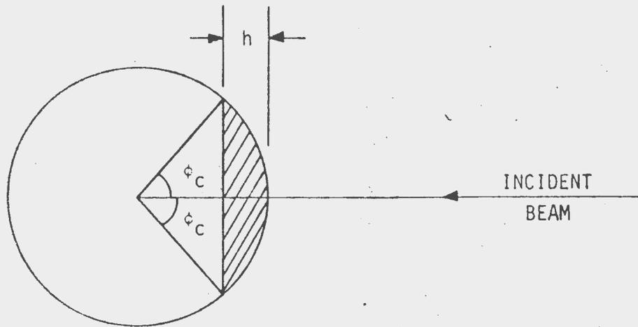
Figure 5. The shaded area is the spherical segment where the "active" cube corners are located when  $\phi_c$  is the cube-corner cutoff angle.
