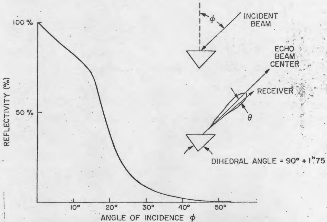
Figure 2. Reflectivity versus angle of incidence for an uncoated fused-silica cube corner with a circular aperture 3.65 cm in diameter and dihedral angles of  $90^\circ + 1.75$  arcsec. The reflectivities are for a beam angle  $\theta$  of  $36\text{-}\mu\text{rad}$ , corresponding to a typical value of velocity aberration for the LAGEOS orbit. The reflectivity is the average for all azimuthal angles (taken around the normal to the front face).
