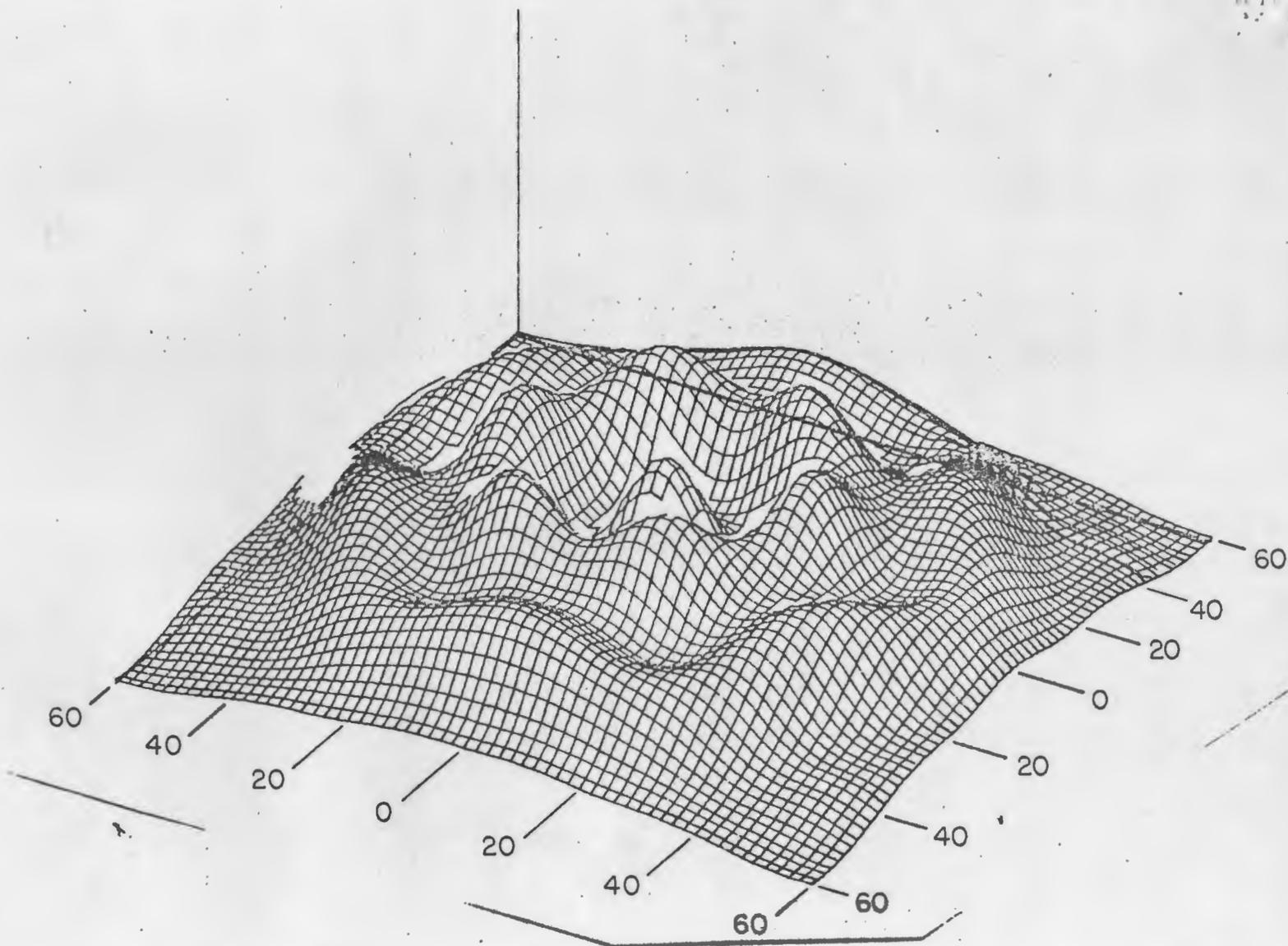
Figure 1. Beam pattern at normal incidence for an uncoated cube corner with a circular aperture 3.65 cm in diameter. Dihedral angle is  $8.5 \mu\text{rad}$  ( $1.57 \text{ arcsec}$ ) from  $90^\circ$ . Beam angles are given in microradians. Wavelength is  $6943 \text{ \AA}$  (ruby laser).
