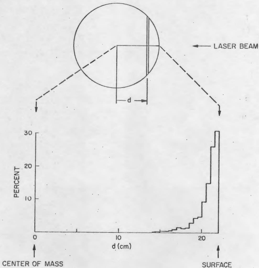
Figure 6. Effective reflectivity of segments of the LAGEOS retroreflector array versus the distance  $d$  from the center of mass. The histogram is the average over results computed for several aspect angles and for incoherent light; i. e., interference effects have been omitted. It is of interest to note that 57% of the total return is from the first centimeter, and 90% from the first 3 cm of the sphere.
